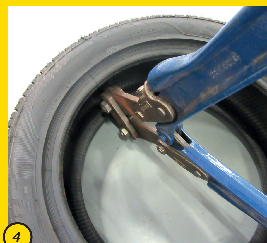
4 Flip tyre over and cut opposite bead bundle.
