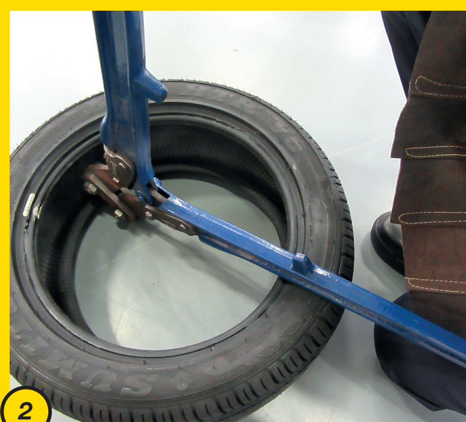
2 Place bolt cutter over bottom bead and cut bead.
