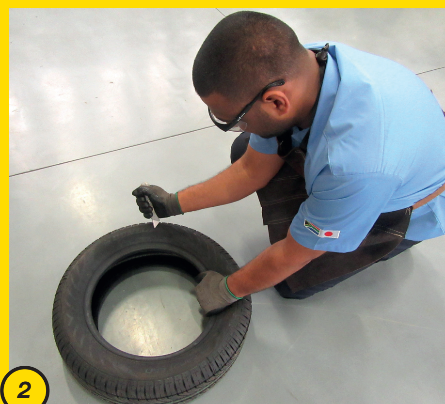
2 Hold bead with one hand. Place knife firmly against sidewall.
