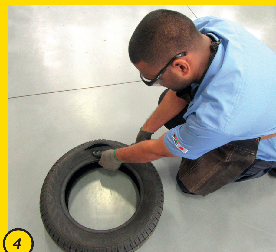
4 Cut sidewall in excess of 100mm circumferentially
