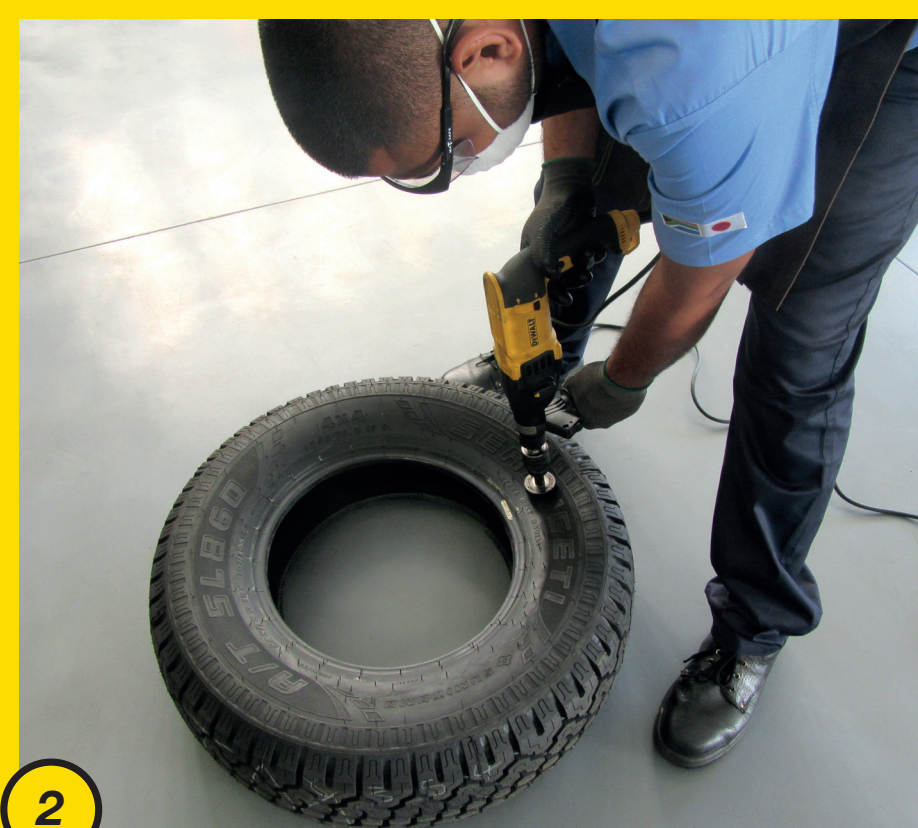
2 Place 50mm hole saw at sidewall region to be cut.
