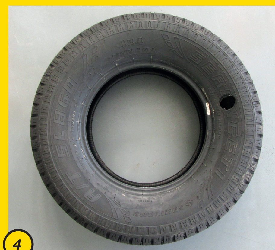
4 Inspect to ensure the hole is completely cut through.
