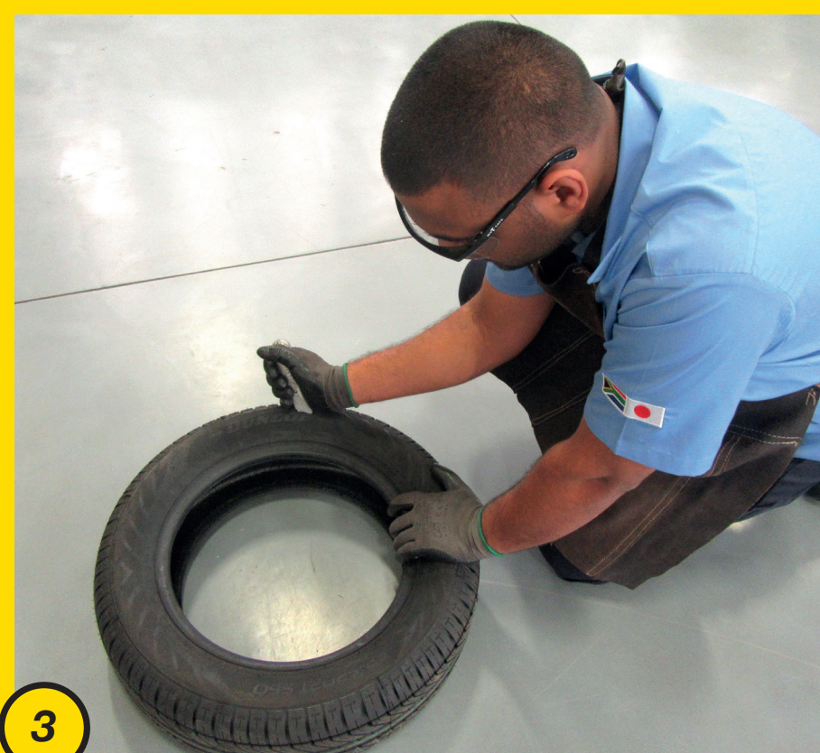
3 Push blade into sidewall while cutting away from body.
