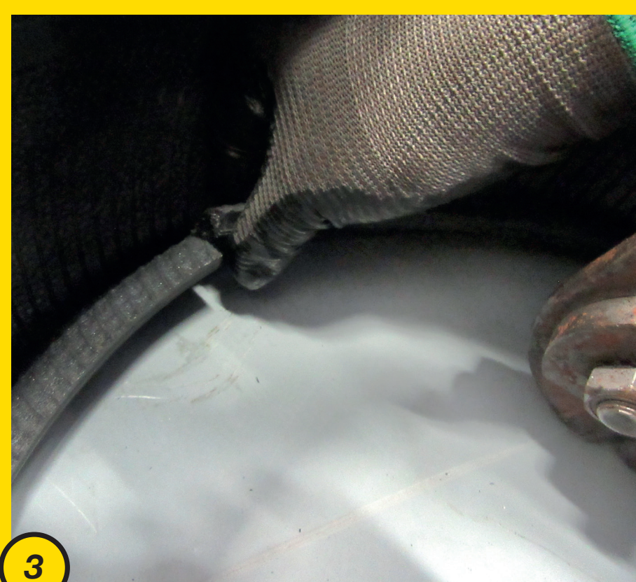
3 Check to ensure that the bead bundle is completely cut.
