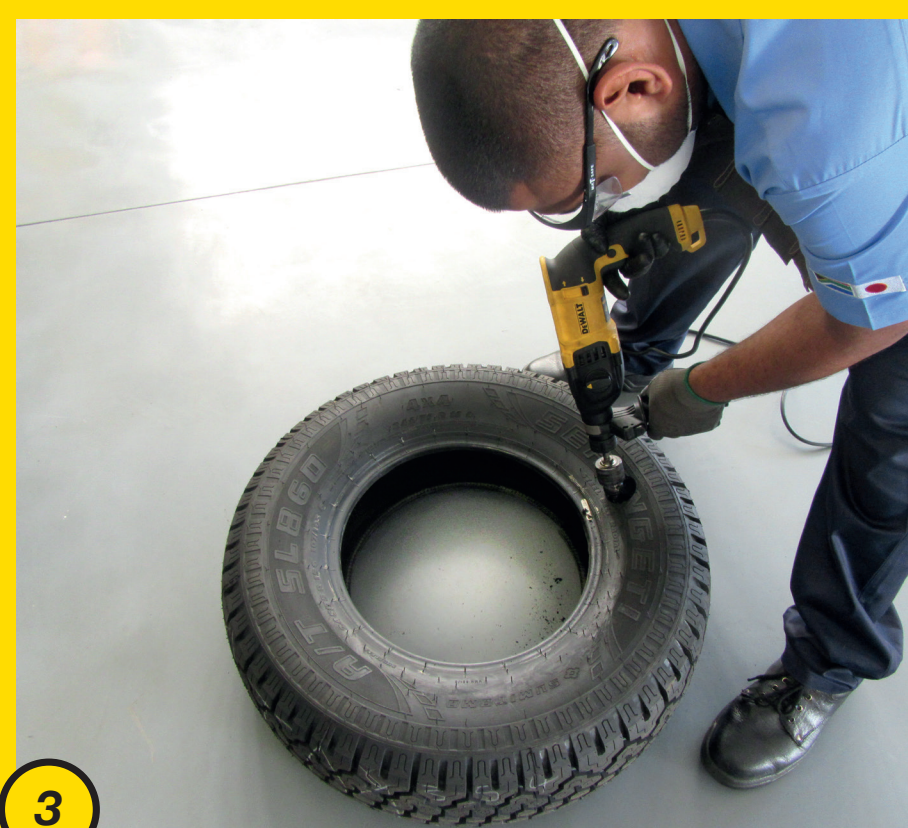
3 Engage drill and cut 50mm hole through sidewall.
